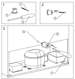
IMPORTANT - THIS SPACER MUST BE ATTACHED TO THE UNIT BEFORE THE INSTALLATION, FOR VENTILATION PURPOSE. FAILURE TO DO WILL VOID THE WARRANTY
